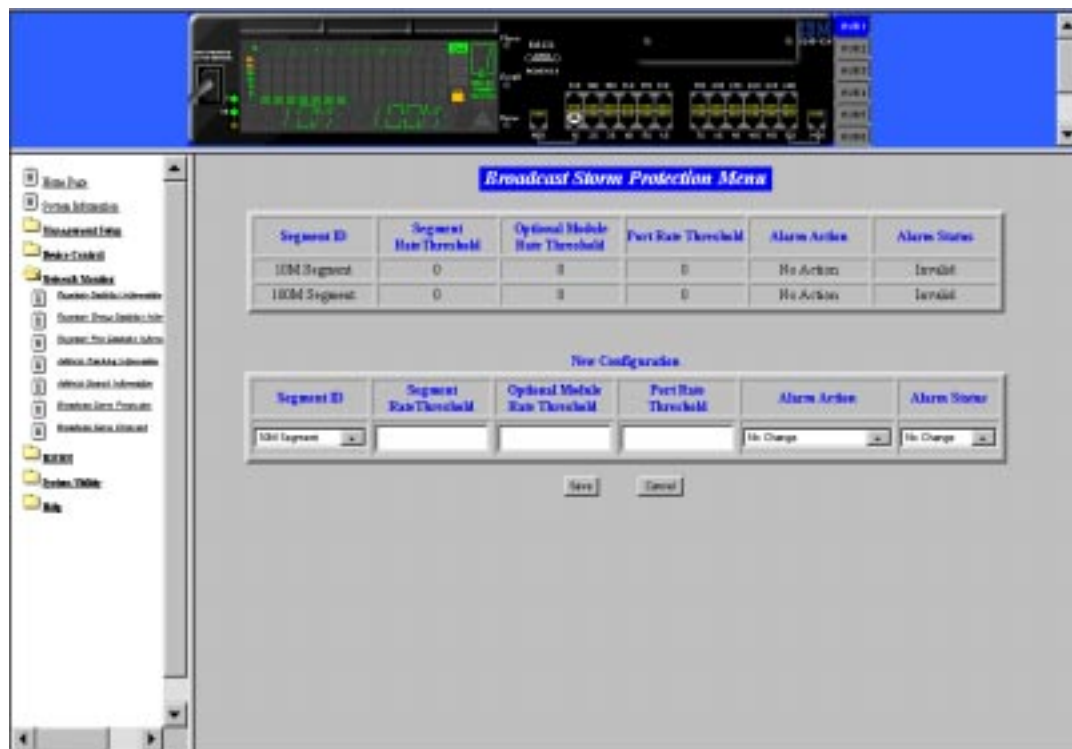
Figure 5-34 Broadcast Storm Protection
