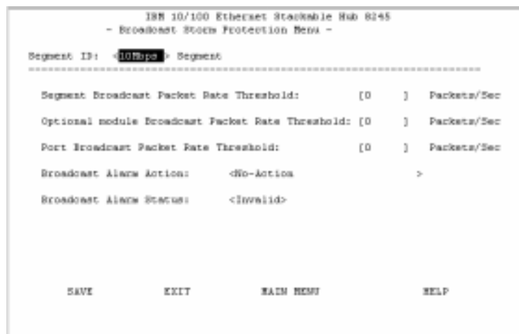
Figure 4-34 Broadcast Storm Protection Menu
